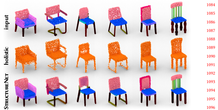
Fig. 8. Reconstruction compared to a holistic approach. We reconstruct the point cloud representation of the shapes in the top row with a holistic approach (orange) that does not use structure, and compare to STRUCTURENET. The holistic approach suffers from noise that results in a loss of detail, whereas reconstruction errors in our approach take the form of slightly modified chair structures, such as the hole added to the backrest in the third column. However, the functional realism of the shape is usually preserved and the explicit structure allows us to preserve significantly more detail.
